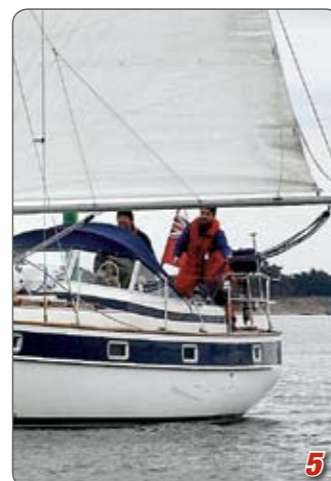
Pics 5 & 6: Easing the mainsail so we can stop the boat in her tracks. Notice how both the falls of the mainsheet and the leech are nice and slack.
