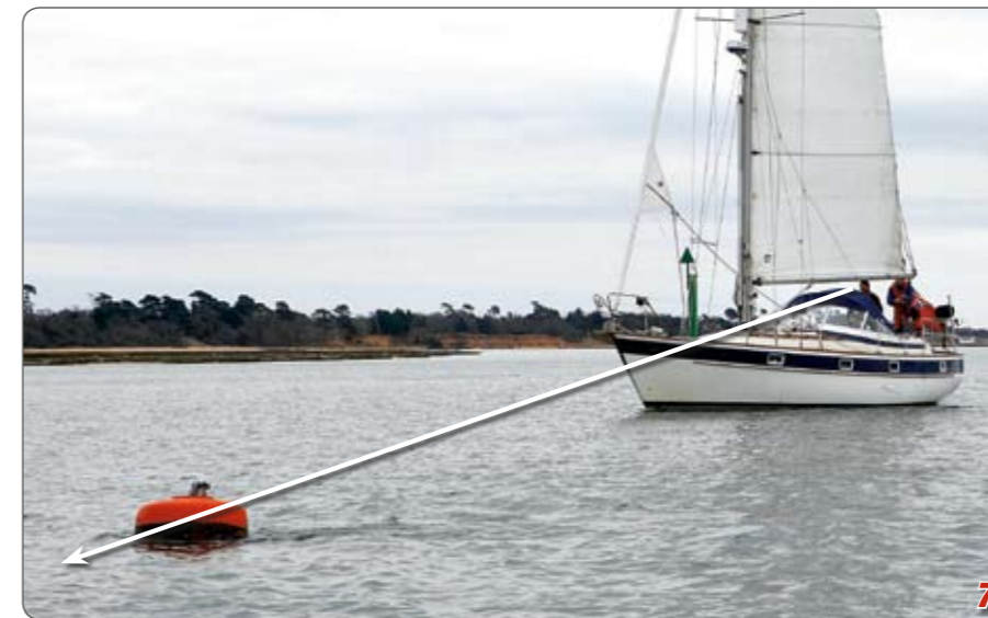
Pic 7-10: With the main de-powered, and having settled on our line of approach we can close gently on the mooring buoy.
