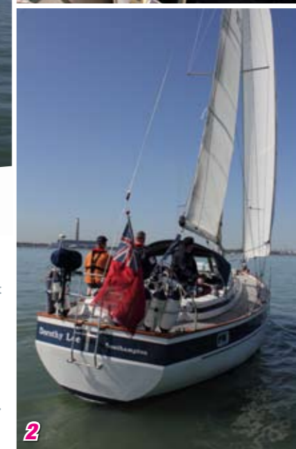
5: Different hull and keel configurations heave to in different ways. In the case of this Hallberg Rassy 352, her displacement and underwater profile lend themselves to a hassle free heave to.
