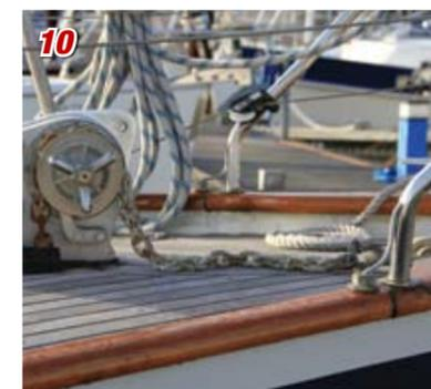
to ready the anchor for deployment we will need to be able to get the chain off the gipsy. With the chain hauled up and allowing a little slack **Pic 7** – you
