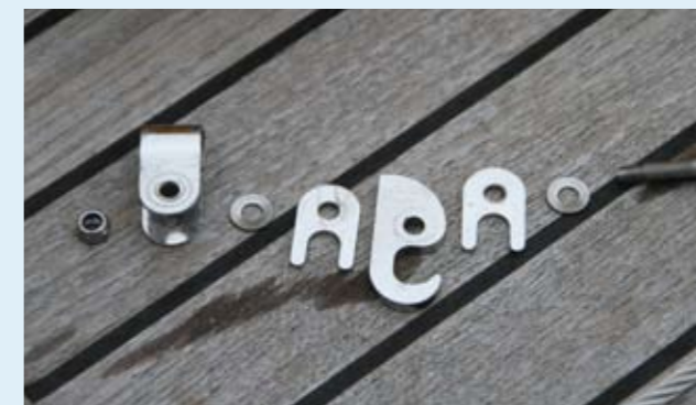
1: The quick release hook assembly.
