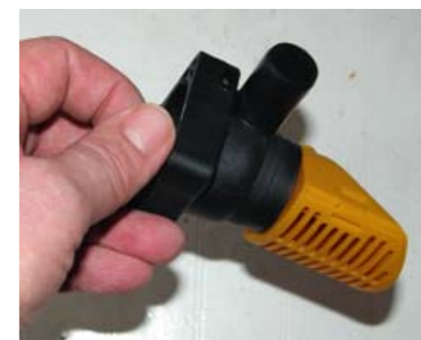
Simply twisting the body allows you to separate the pump motor.
