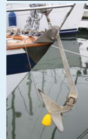
3: Be careful the wire and float do not foul the bow roller cheeks as you drop anchor.
