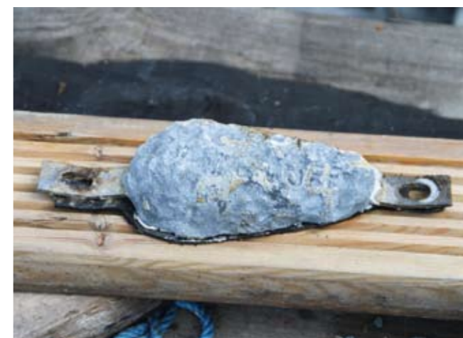
Plenty of the anode left after 14 months.
