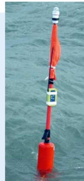
Being January, with a water temperature of just 6°C, we were reluctant to put a man in the water for any length of time, so we tested the beacon by attaching it to a floating Dan buoy – mounting it so it would simulate being held up by someone wearing a lifejacket and floating in the water a couple of feet above sea level.
