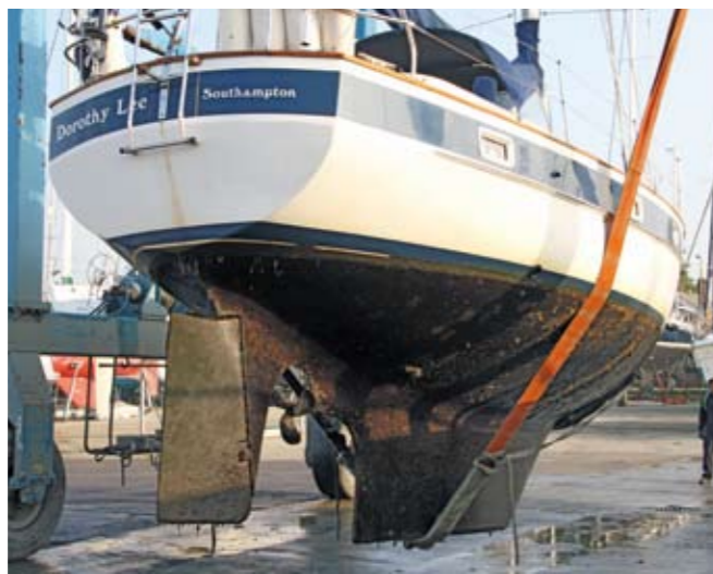
The hull after 14 months in the water with six year old CopperPlus.
