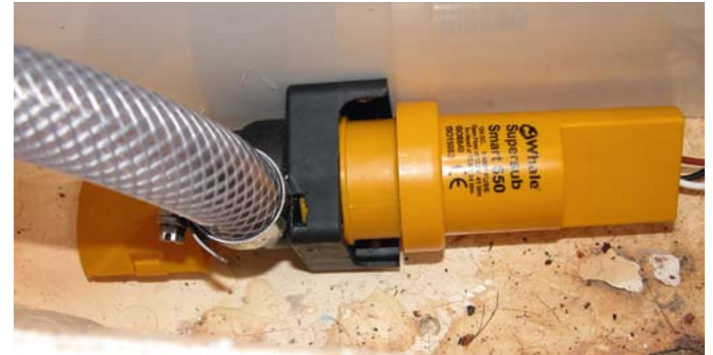
Compact and easy to install, the Whale Supersub 650 shifts a healthy 32 litres per minute.
