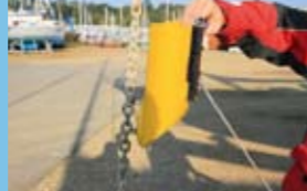
As the end of the wire is lifted, so it releases from its clip.
