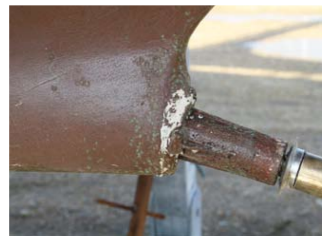
The CopperPlus had worn away in a couple of places.
