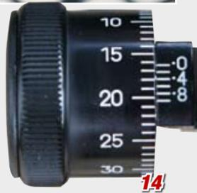
are slightly out, so .4 it is and the angle of the sun at the time we took the sight was 41° 16'.4. And there is nowhere that I have ever come across that has explained how to read the arc and micrometer scale like that – a way that means you can actually do it.
