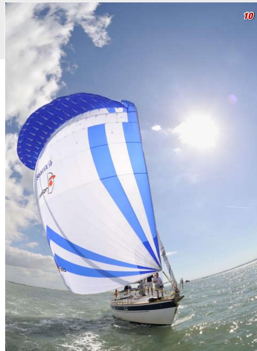
Setting the Parasailor in light airs was a breeze. The sail is remarkably light and colour coding on the clews means you are less likely to get in a tangle when hoisting with the help of a snuffer.
