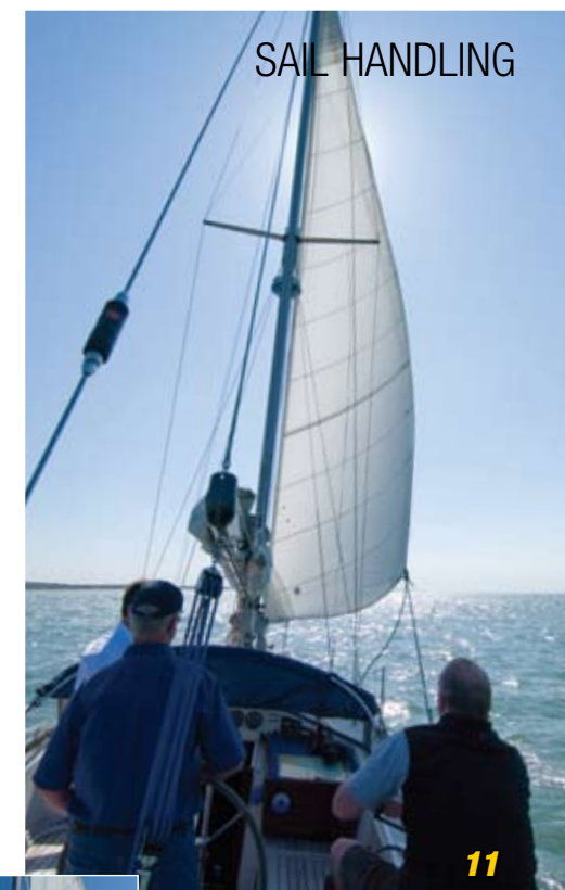
11 Closehauled on port. 12 Sheet eased to depower sail and allow the momentum to take us through the wind. 13 Headsail backed. 14 Round she goes.
