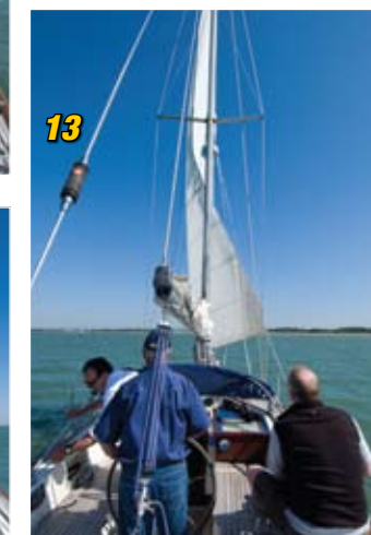
11 Closehauled on port. 12 Sheet eased to depower sail and allow the momentum to take us through the wind. 13 Headsail backed. 14 Round she goes.
