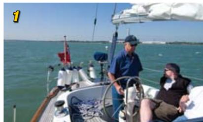
1 Head to wind – notice how the power station chimney is in line with the helmsman
