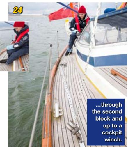
24 ...through the second block and up to a cockpit winch.
