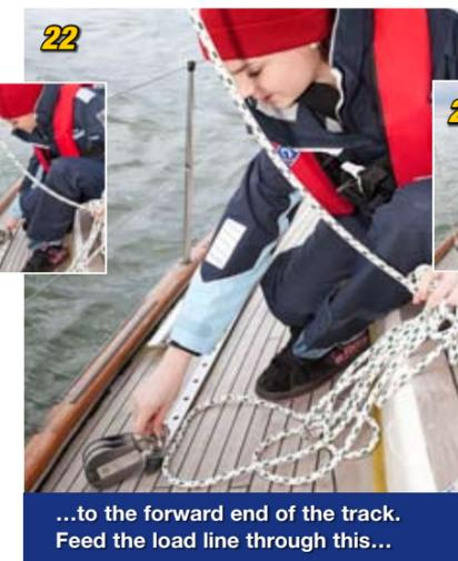
22 ...to the forward end of the track. Feed the load line through this...
