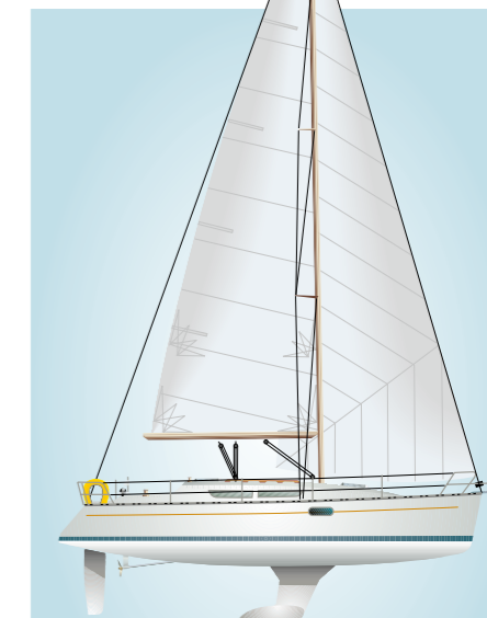
Jeanneau Sun Odyssey 36i Short fin keel and spade rudder Marc Lombard
