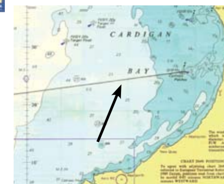
6 On this chart of 1:500,000 scale this 1mm pencil line is 500 metres wide.
