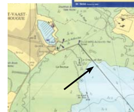
5 On this chart of 1:20,000 scale this 1mm pencil line is 20 metres wide
