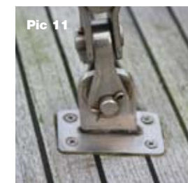
Pic 11: Split pin back in place and bent back. Pic 12: All in order on Dorothy Lee as she sets sail again.
