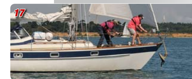
14. The weight of the boat is taken gently off the chain. 15. The hauler and a crew member tailing. 16. Over running the anchor slightly to help break it out. 17. Up she comes, covered in mud.
