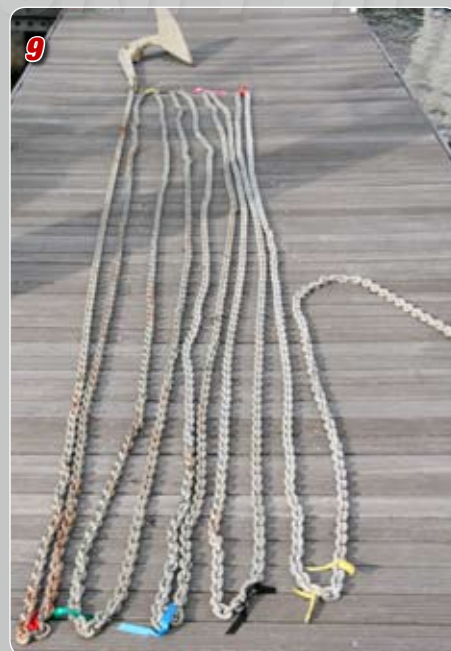
We marked the chain with coloured silks at 5m intervals: Red 5m, Yellow 10m, Green 15m, Brown 20m, Blue 25m, Pink 30m, Black 35m, 2 x Red 40m, 2 x Yellow 45m (we have 50m of chain) Pic 9.
