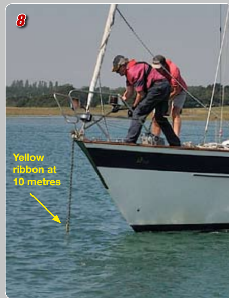
We marked the chain with coloured silks at 5m intervals: Red 5m, Yellow 10m, Green 15m, Brown 20m, Blue 25m, Pink 30m, Black 35m, 2 x Red 40m, 2 x Yellow 45m (we have 50m of chain) Pic 9.
