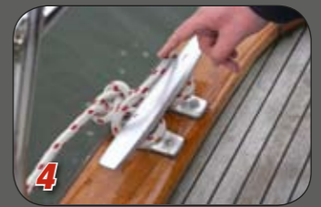
4 ... and then looping it over each wing, with the line ...
