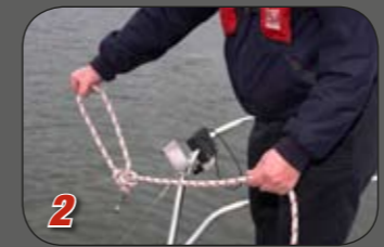
2 Bowline with snap shackle at inboard end of the line.
