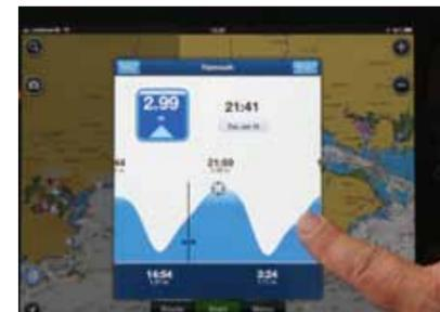
The popular Navionics app includes tidal times and heights, as well as tidal flow direction and speed
