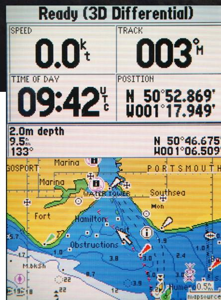
**Augmentation systems improve GPS accuracy by comparing our position with that of known objects and applying an offset**
